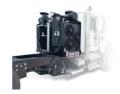
he BOSSAIR 900 is the most unique rotary screw air compressor package on the market today. When the job demands the most out of the vehicle, the BOSSAIR 900 is the only choice for the largest jobs. Utilizing two rotary screw air compressors, driven off two separate PTOs to produce the maximum mobile air compressor performance available on a single Class 8 type platform.
